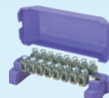
EB 16 Art.-No. 690 005 For connection of the earthing conductor of various equipment or system. This bars have 16 connecting terminals, with 8pcs max. cross-section area 25mm 2 , and 8pcs max. cross-section area 50mm 2 .
